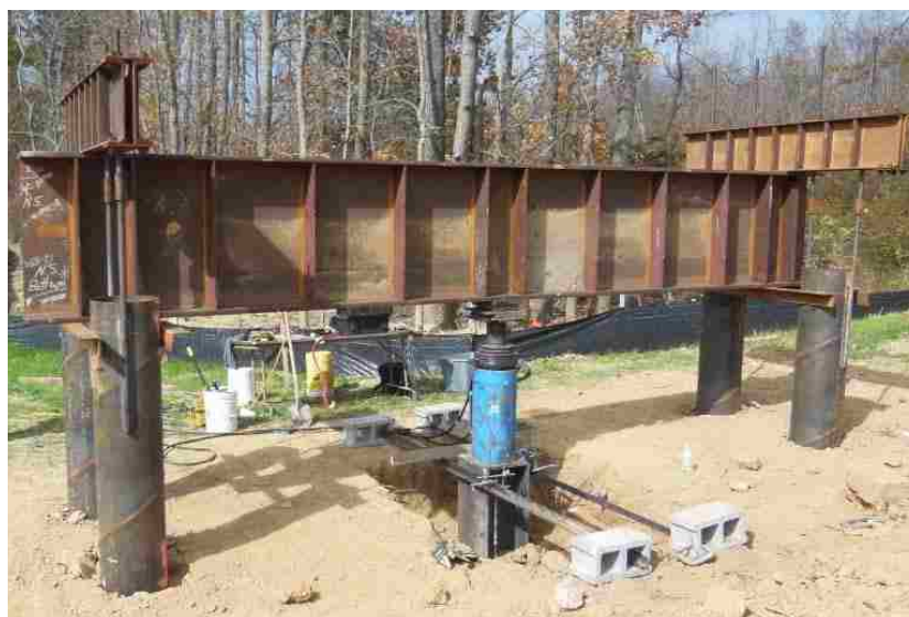
Figure 5.23 Completed A7669 Pile Load Test Set-up
